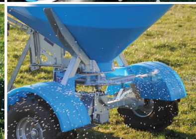
Stainless steel spinner disc with adjustable spinner fins
